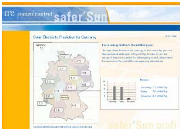
Figure 6: Screenshot of the web-based graphical user interface showing daily sums of PV electricity production normalized to the total installed capacity for each German federal state and the whole country.
